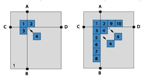
When laying on raised floor subfloor, the tiles are aligned in a form identical to the raised floor plates (generally 60 x 60 cm) as per the existing raised floor pattern. The centre axes of tiles are aligned on the joints of the raised floor plates. Thus, a tile generally rests on each of the four raised floor plates.
